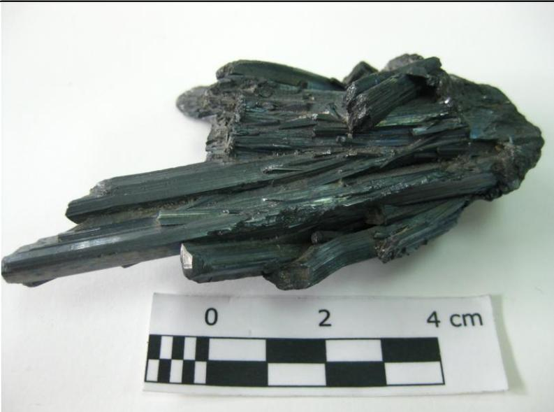
A photograph showing a cluster of dark, metallic, acicular (needle-like) stibnite crystals. The crystals are elongated and have sharp, pointed ends. They are attached to a dark matrix. Below the specimen is a scale bar with markings at 0, 2, and 4 cm.                                |
