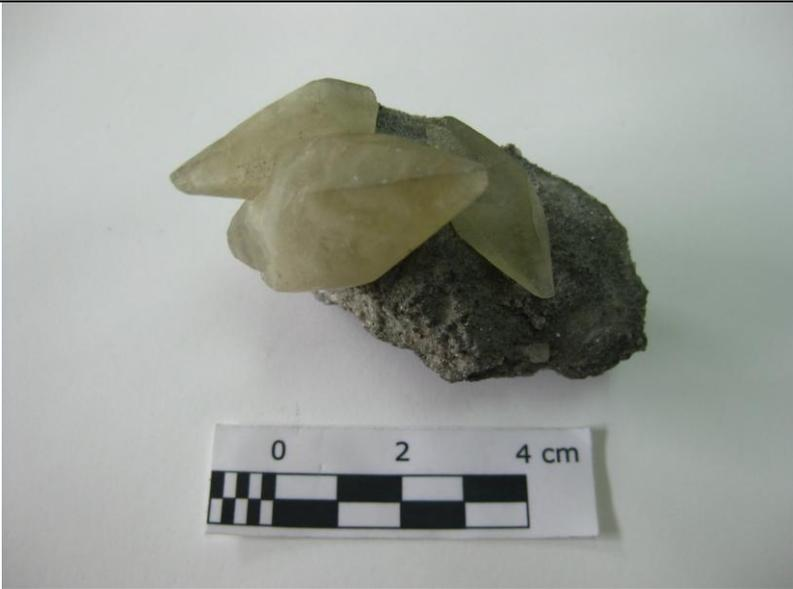
A photograph showing several translucent, yellowish, scalenohedral calcite crystals. The crystals are idiomorphic and have a characteristic three-sided, flat-topped shape. They are attached to a dark, greyish matrix. Below the specimen is a scale bar with markings at 0, 2, and 4 cm. |
